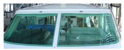
Perimeter painted frit is a colored band on glass applied during the manufacturing process that serves as a barrier against UV radiation to protect the adhesive. It also provides a cosmetic benefit by concealing the adhesive when viewed from the outside. Typically, the frit is black, but white can also be an option.
