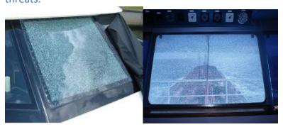
A second issue with tempered glass is distortion that can occur in manufacturing. This distortion is often distracting to the viewer. In extreme cases, distortion in tempered glass can cause the person looking through the glass to feel sick and dizzy. Chemically strengthened glass is not subject to optical distortion, thus, eliminating the possibility of these effects.
