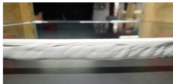
Image 3 – Abraded and cleaned edge seal surface
